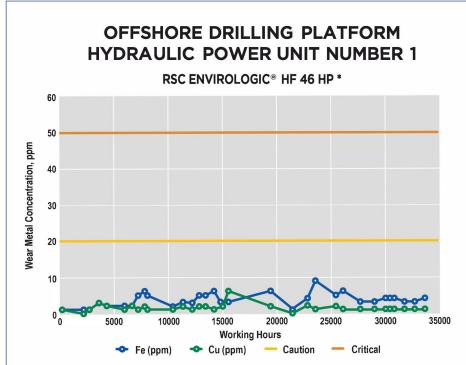
(Top) Plot of the results from a sample industry in-service oil analysis, showing condition monitoring according to ASTM D664. In comparison are the performance of HEES and RSC EnviroLogic HF 46 HP (formerly EnviroLogic 3046). (Bottom) Sample data from an offshore drilling platform showing wear metal concentration. The level of iron and copper never approached the caution threshold during all measured hours of operation using RSC EnviroLogic HF 46 HP (formerly EnviroLogic 3046).
